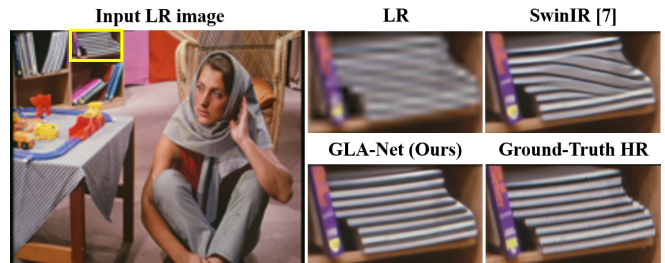
Fig. 1. Visual comparison with state-of-the-art SwinIR [7] at 4\times super-resolution. Our GLA-Net is more effective at recovering local details, such as edges, than SwinIR.
